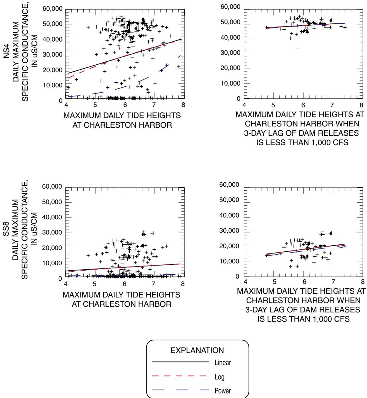
Figure 23. Maximum daily tide height at Charleston Harbor with daily maximum specific conductance at NS4 and SS8 for the entire range of dam releases and dam releases less that 1,000 cfs.
