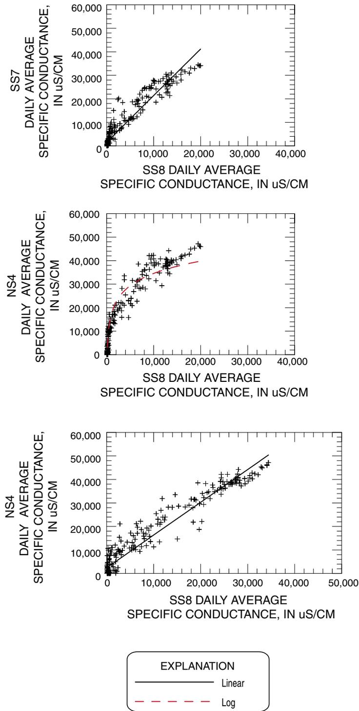
Figure 21. Regression analysis plots of daily average specific conductance between NS4 and SS7, NS4 and SS8, and SS7 and SS8.
