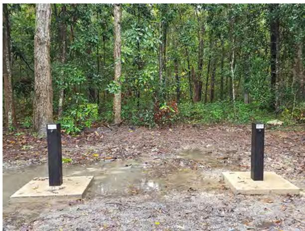
**Figure 19. New monitoring wells at Myrtle Beach State Park in Horry County. HOR-1326 (left) is screened in the McQueen Branch aquifer (600 feet deep) and HOR-1327 (right) is screened in the Crouch Branch aquifer (440 feet deep). HOR-1327 is also part of the Saltwater Intrusion Monitoring Network.**
