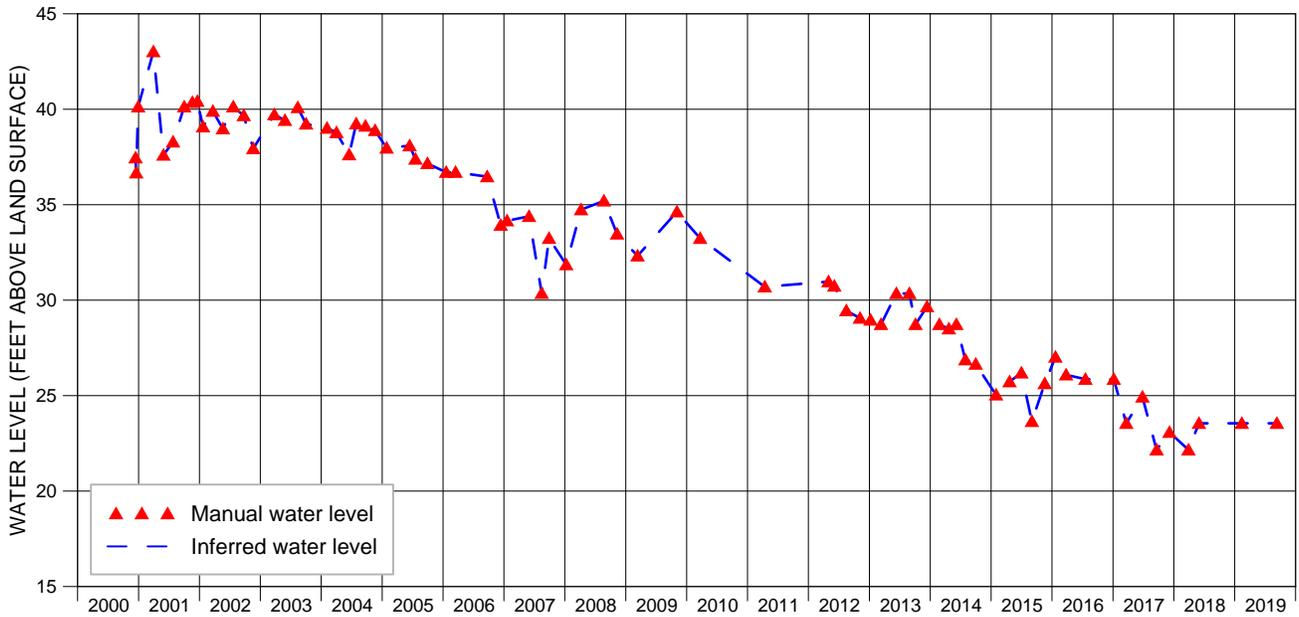
**Figure 11. Manual water-level measurements in well MRN-0078 (Marion County). Because the water level in this well is above land surface, an ADR is not used, and measurements are made using a pressure test gage.**
