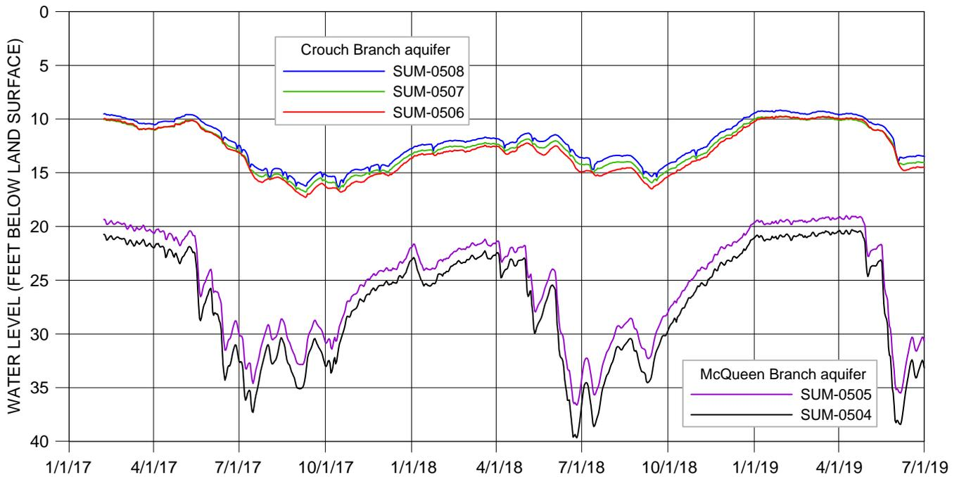
**Figure 24. Daily average water levels measured in the five network wells at the Sumter cluster site in Sumter County. The seasonal water level declines observed during the summer each year are the result of local groundwater pumping for agricultural irrigation.**
