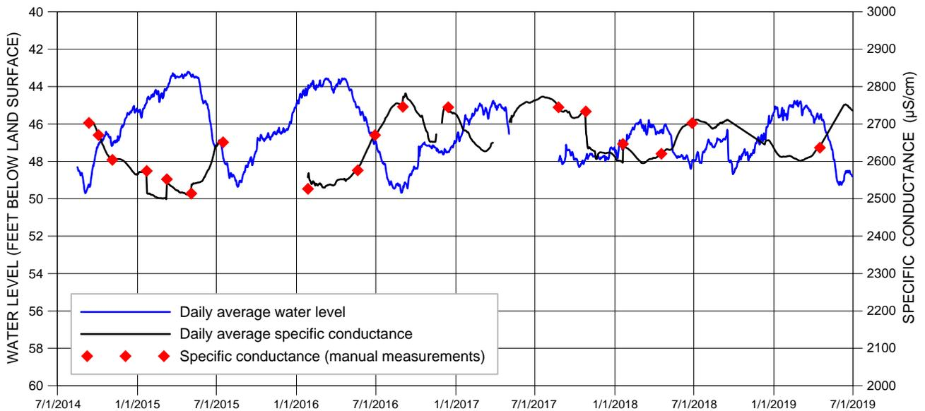
**Figure 12. Daily average water level and specific conductance for the Gordon aquifer well CHN-0989 in Charleston County. Manual measurements of specific conductance made during site visits verify the accuracy of the ADR data.**
