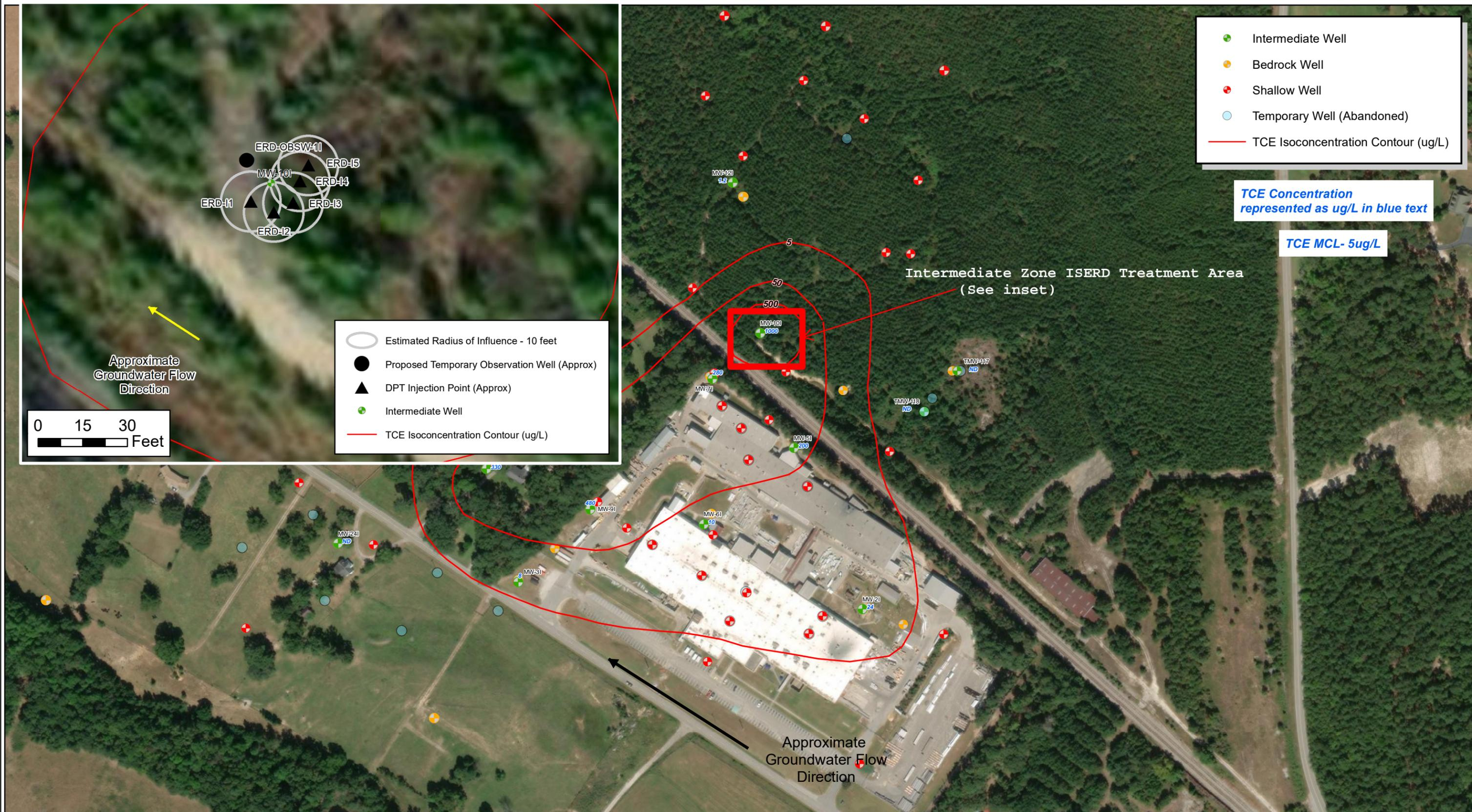
Figure 4 : Enhanced Reductive Dechlorination Pilot Study Area (ISB and ISCR) - Intermediate Zone
