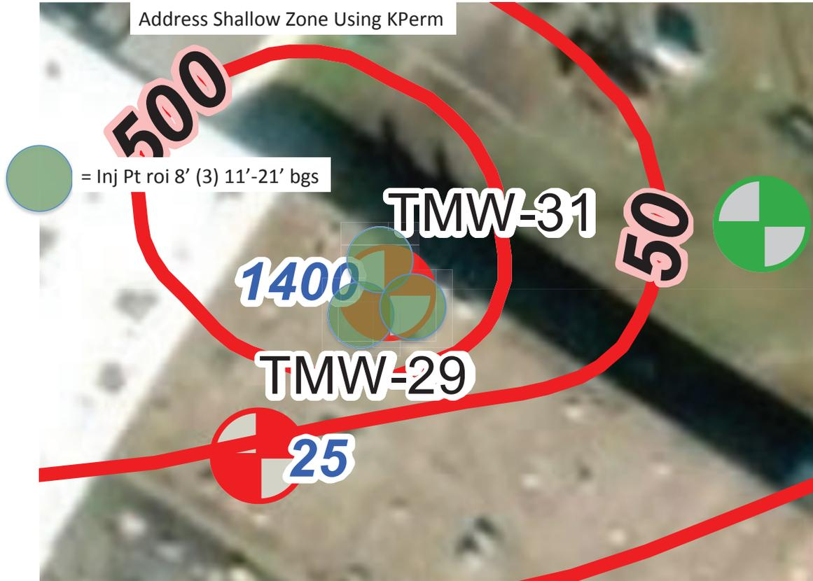
**Figure 1. Potassium Permanganate Injection Location Map**
