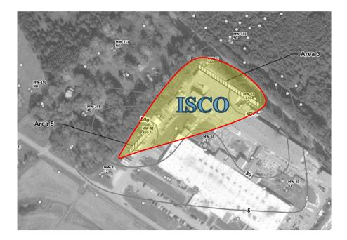
In Situ Chemical Oxidation (ISCO), In Situ Enhanced Reductive Dechlorination (ISERD), In Situ Adsorption (ISA), Monitored Natural Attenuation (MNA), Institutional Controls (IC), and Containment via Cover (CvC)
