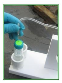
5. Connect a <u>new extraction needle</u> assembly to the colorimetric tube by sliding the open end of the vinyl tubing over the broken end of the colorimetric tube. This step must be completed before inserting the needle into the VOA (Prior to step 6).
