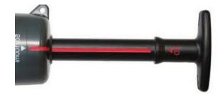
14. Continue the 100ml purge until the flow cycle is complete. Note: Flow is complete when the end-of-flow indicator (located on the back of the pump handle) returns to its full brightness.
