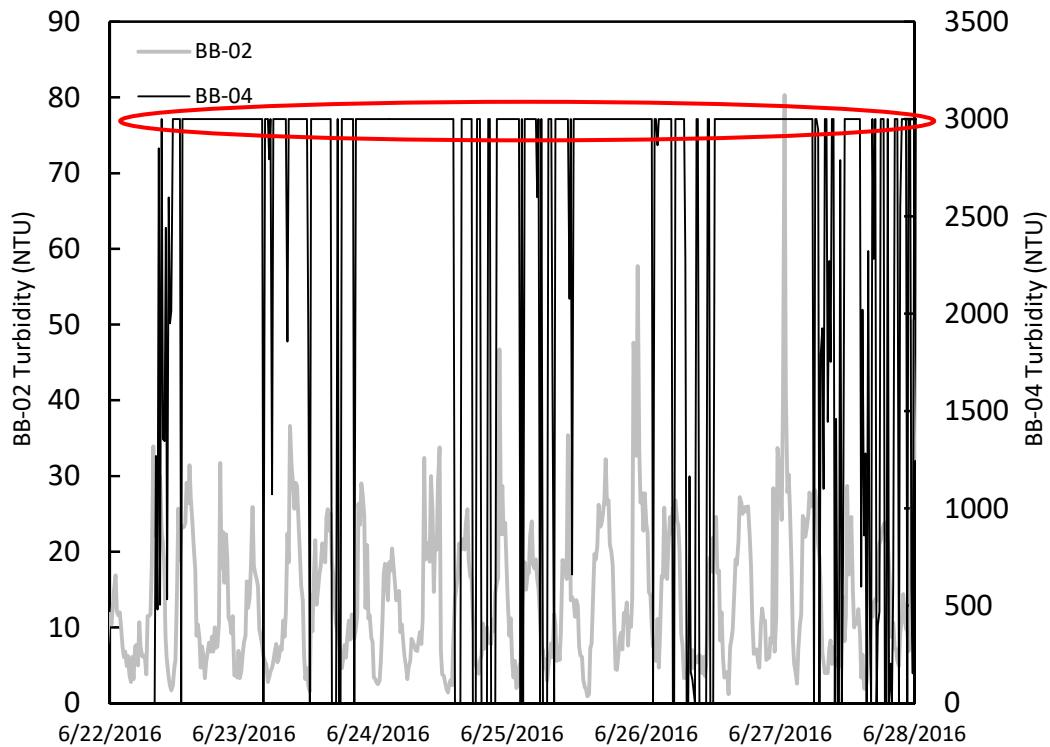
Continuous monitoring Turbidity data from within the same field area. The record from Station BB-04 site is the result of turbidity sensor failure during deployment and is typical of obviously erroneous data. Please note the extreme difference in Turbidity scales between the primary and secondary vertical axes as well as the flat shape of the BB-04 profile across the top highlighted by the red circle.
