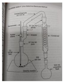
Image 1.0 Distillation Apparatus per SM 4500.
