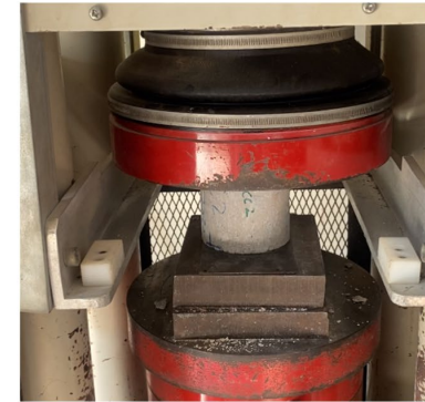
Mount concrete specimen in machine
