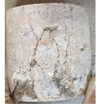
Compress the specimen until it fails
