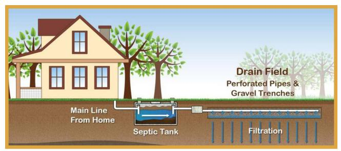
Figure 3.7 Diagram of a septic system (Minnesota Pollution Control Agency 2023)
