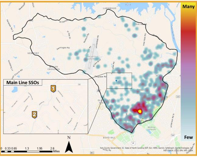
Figure 3.5 Main line SSOs (points 1 and 2) and service line SSOs (heat map) in watershed
