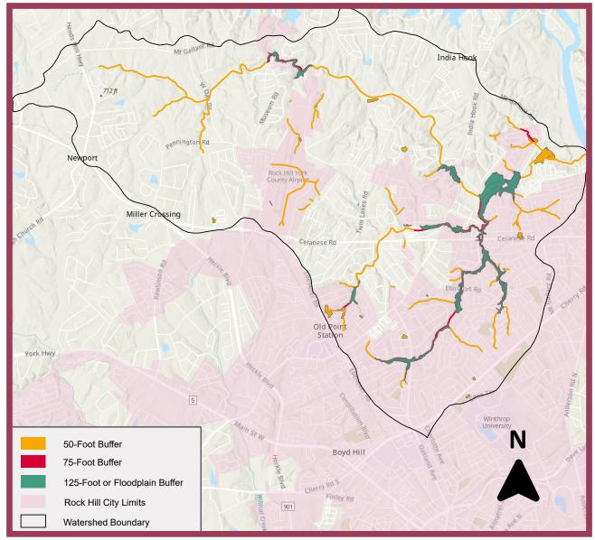
Figure 1.14 Stream buffer limits in watershed
