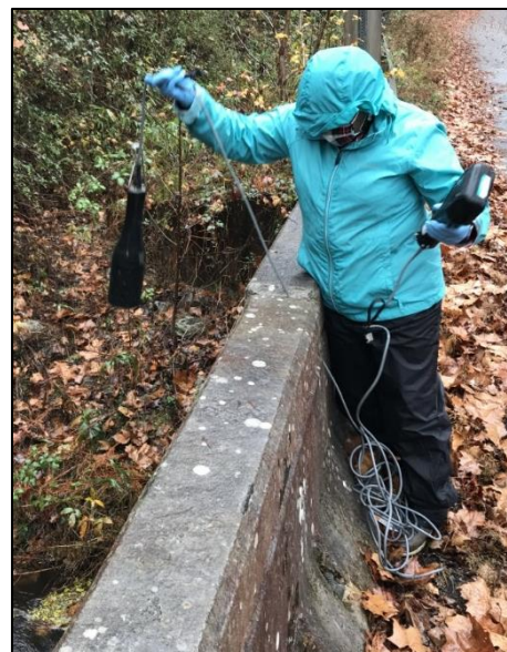
Using a Horiba Water Quality Meter to determine field parameters
