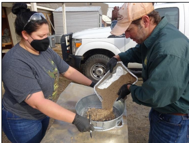
Pieces of rockier sediment are sieved before samples are sent to the Columbia lab for radionuclide analysis
