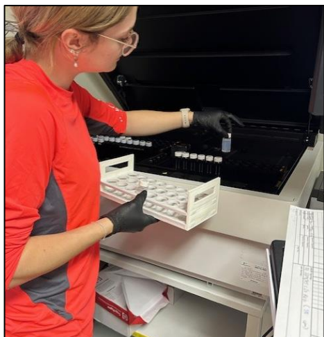
Preparing for tritium analysis in a Liquid Scintillation Counter
