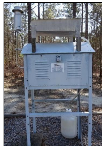
Example of an Air Monitoring Station with Rain Collection Pan and Glass Fiber Filter (on top) and Silica Gel Column (inside)
