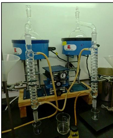
Collecting atmospheric moisture from silica gel through distillation
