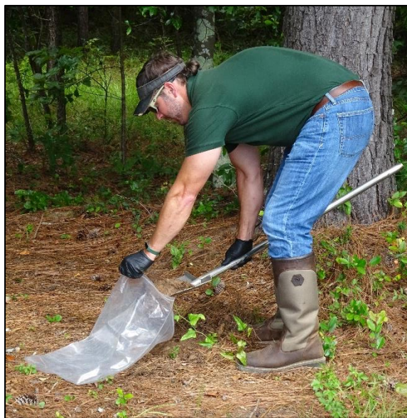
Collecting soil samples which will be analyzed for radiological material and metals
