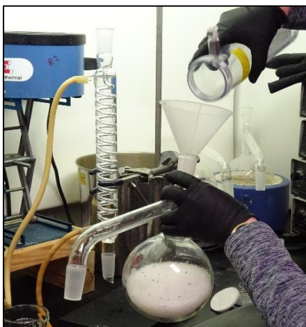
Collecting atmospheric moisture from silica gel through distillation
