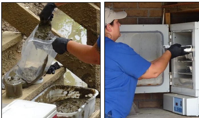
Sediment is collected and then dried before radiological analysis
