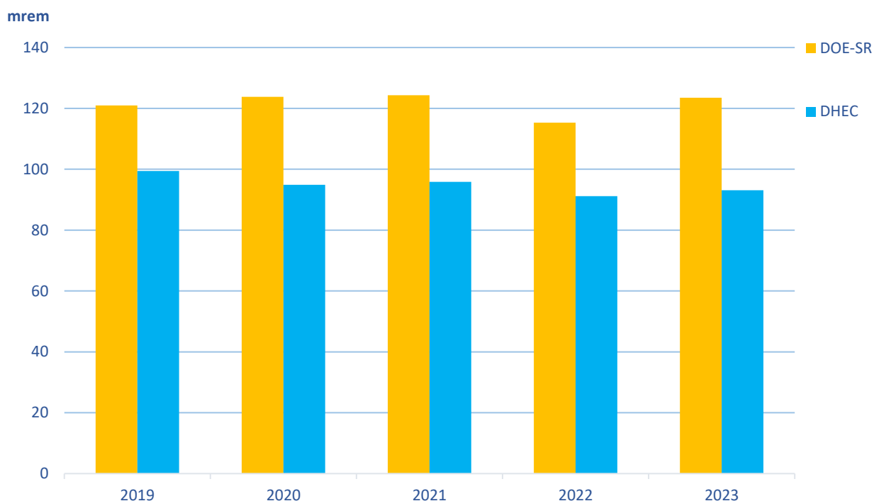
Figure 3. 2019-2023 DOE-SR and DHEC Comparison of Yearly Average Ambient Beta/Gamma Dose for Dosimeters at the SRS Perimeter (SRNS, 2020-2024; DHEC, 2020-2023)
