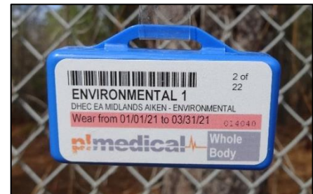
Example of dosimeters present at 19 locations
