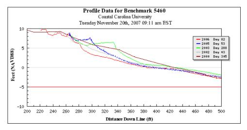
Stations 5470 - 5480 are located in the northern commercial district, although there are several residential structures here as well. A small but well-defined primary dune exists along most of the beach. Surveys show the beach profile here to be eroding during the survey period similarly to the section to the south, with accumulation of sand between -5 and -10 ft.
