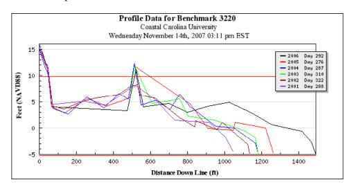
Along the developed southern half of Dewees, station 3220 showed significant accretion through October 2006. Stations 3230, 3250, and 3255 all experienced some erosion at the seaward end of the profile, between the 0 and -5 ft contours, but maintained a net increase in sand across the entire profile. Station 3240 has experienced continuous loss in the profile since 2002, with a landward shift in the berm between 2004 and 2005 and relative stability into October 2006.
