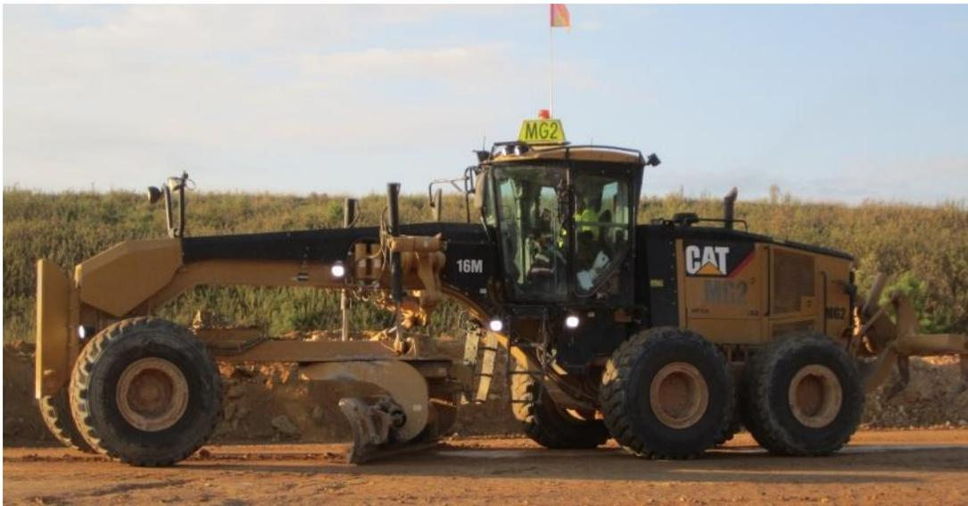
**Figure A-14** Motor Grader
