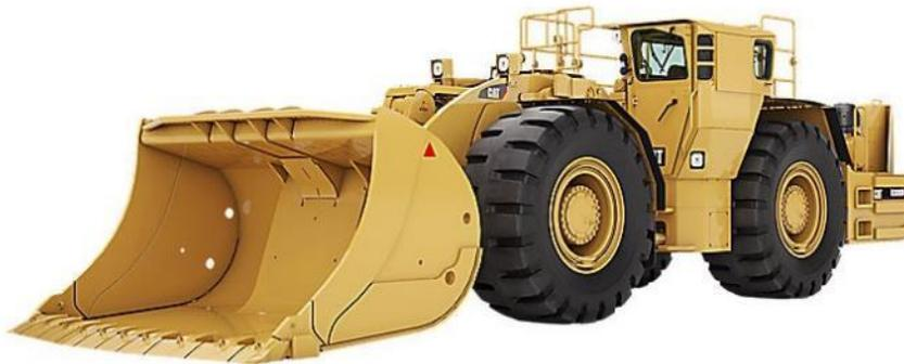
**Figure A-34 Typical Load-Haul-Dump (LHD) Unit**
