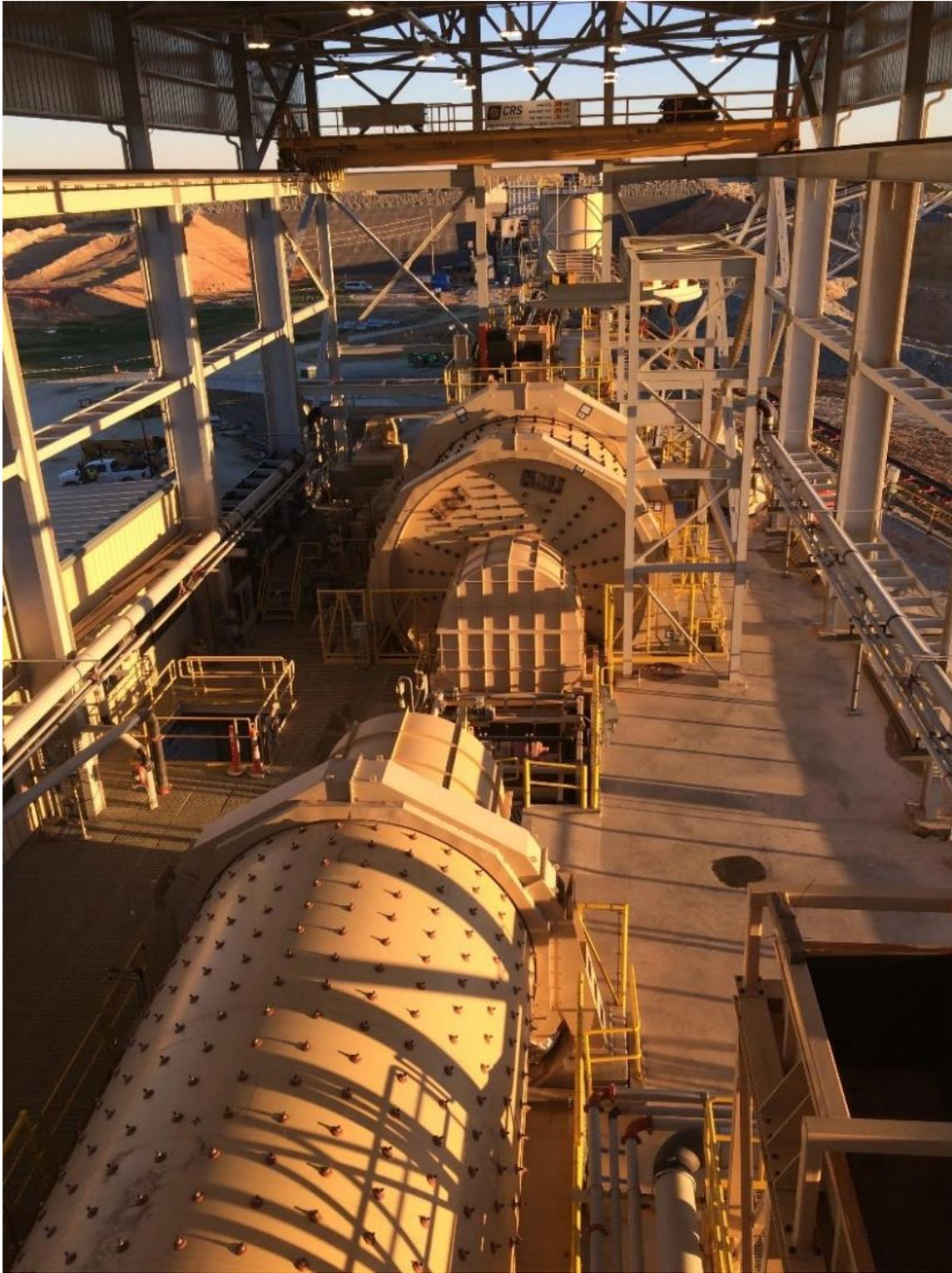
**Figure A-45 Grinding Circuit – SAG Mill and Ball Mill**
