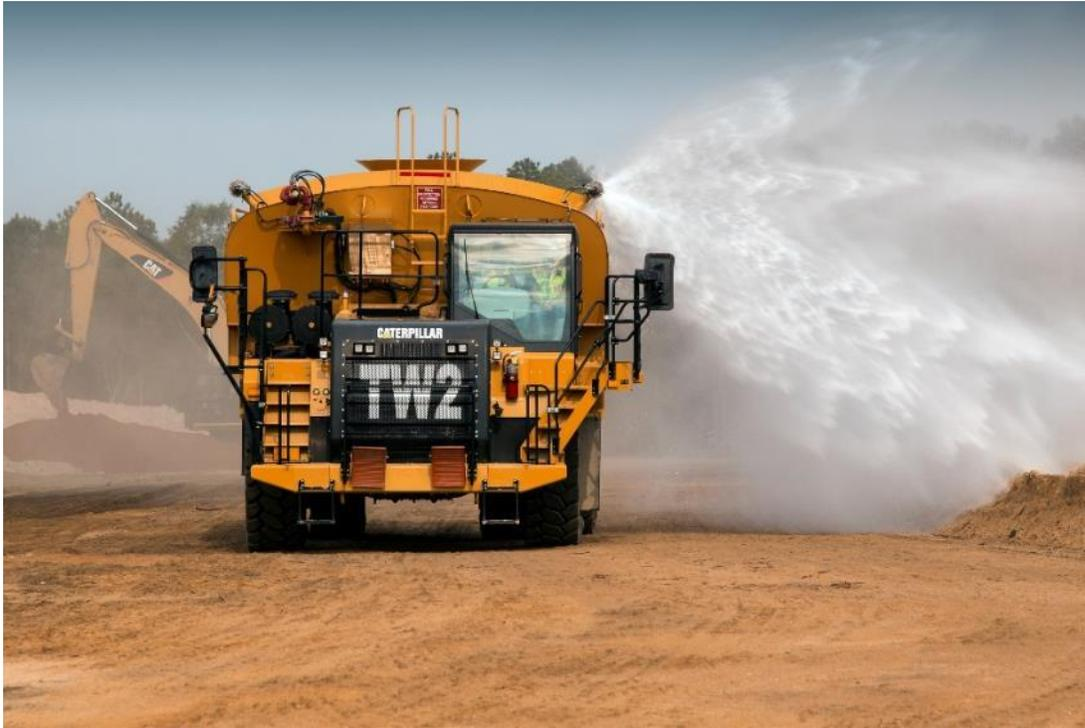
**Figure A-15 Water Truck for Dust Control**
