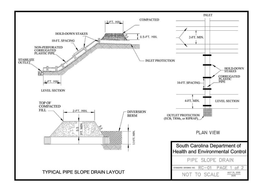
PIPE SLOPE DRAIN
