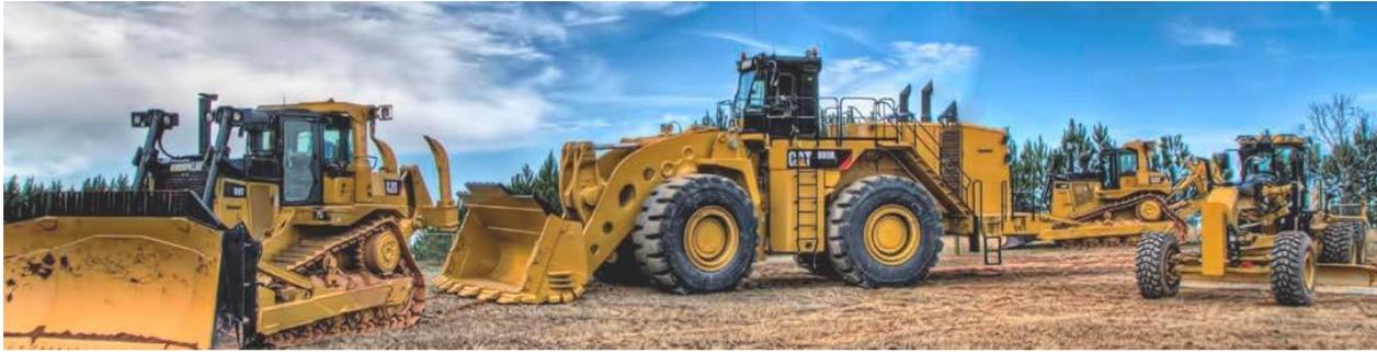
**Figure A-13** Example of a Track Dozer (left and in background), Wheel Loader (center), and Motor Grader (far right)
