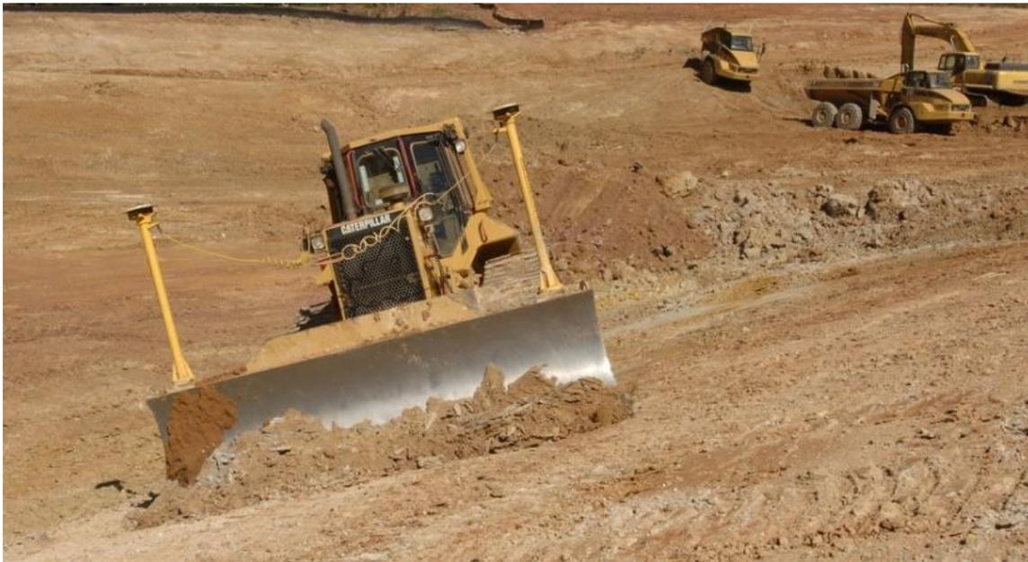
**Figure A-16 Dozer with GPS Controls (Foreground), Articulated Trucks and Excavator (Background)**
