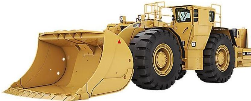
**Figure A-34 Typical Load-Haul-Dump Unit (LHD)**
