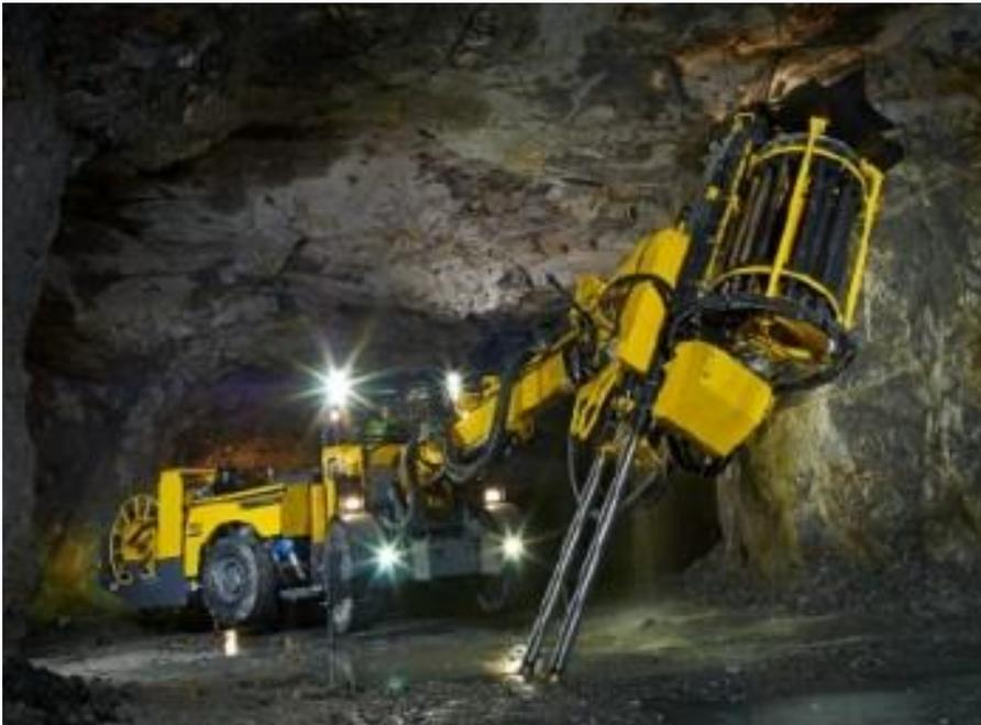
**Figure A-35 Typical Down-the-Hole (DTH) Drilling Unit**
