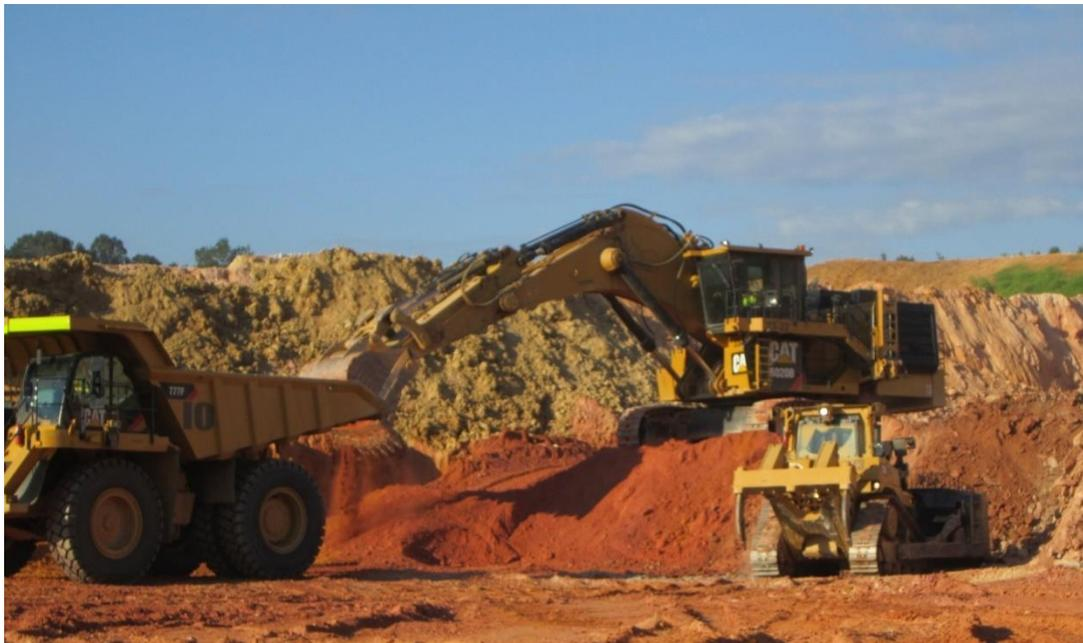
**Figure A-12 Hydraulic Excavator, Dozer, and Haul Truck**
