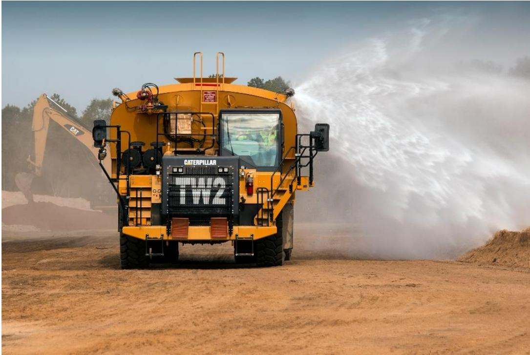
**Figure A-15 Water Truck for Dust Control**
