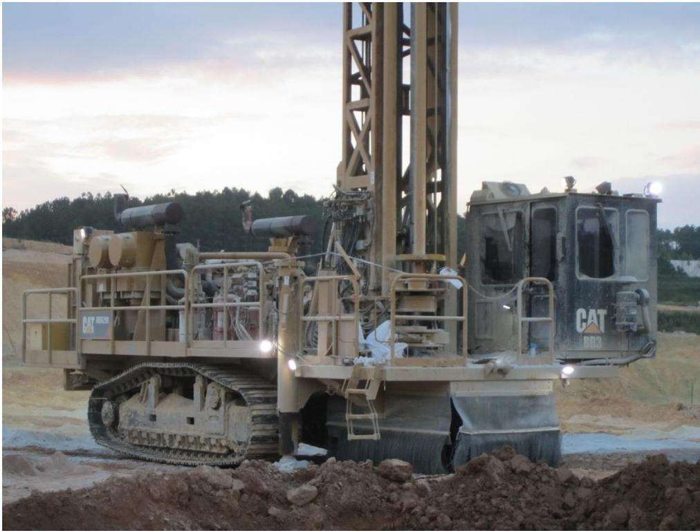
**Figure A-10 Blast Hole Drill**
