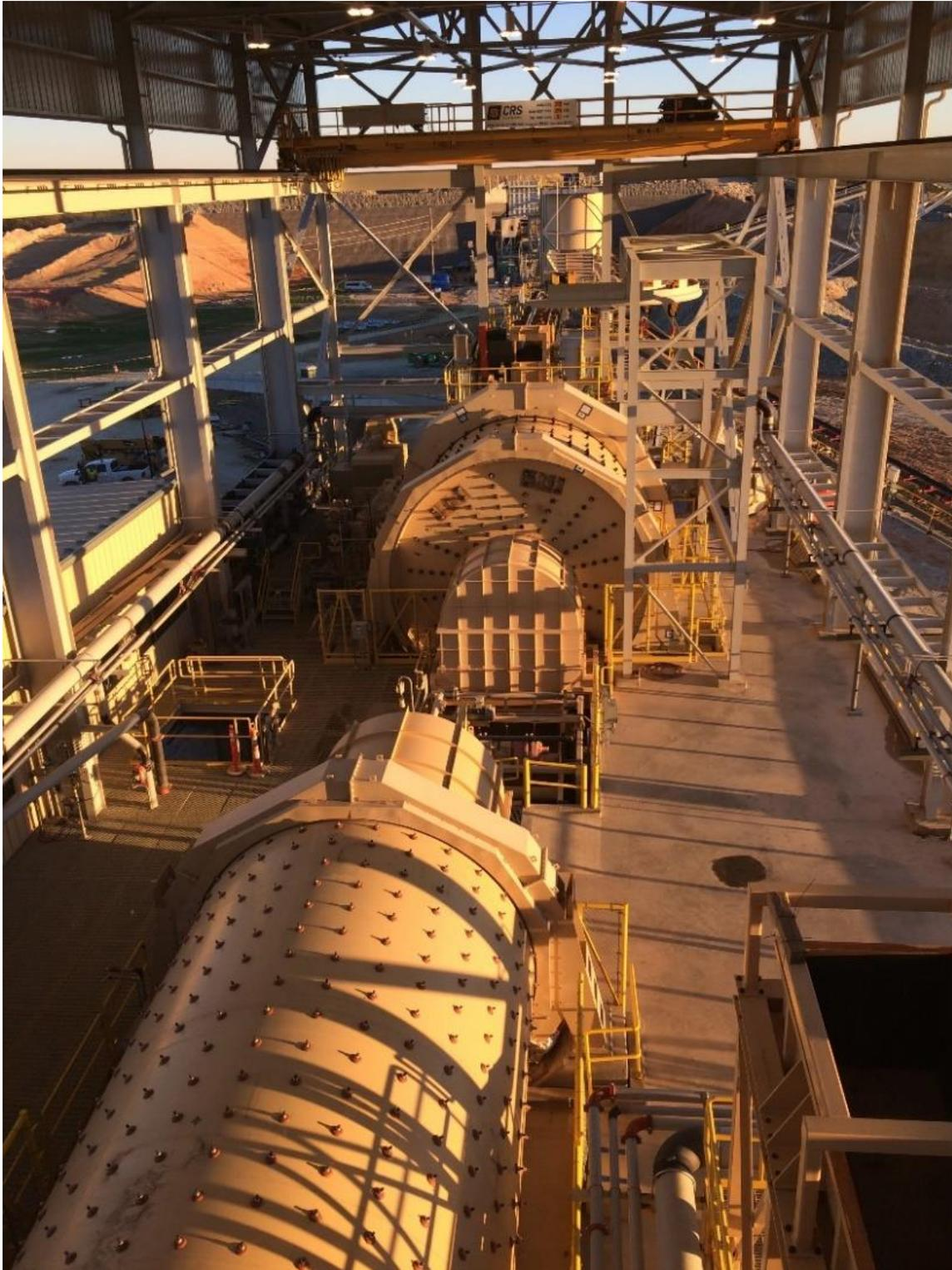
**Figure A-47 Grinding Circuit – SAG Mill and Ball Mill**
