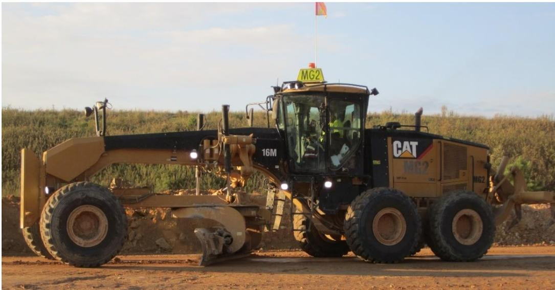
**Figure A-14** Motor Grader
