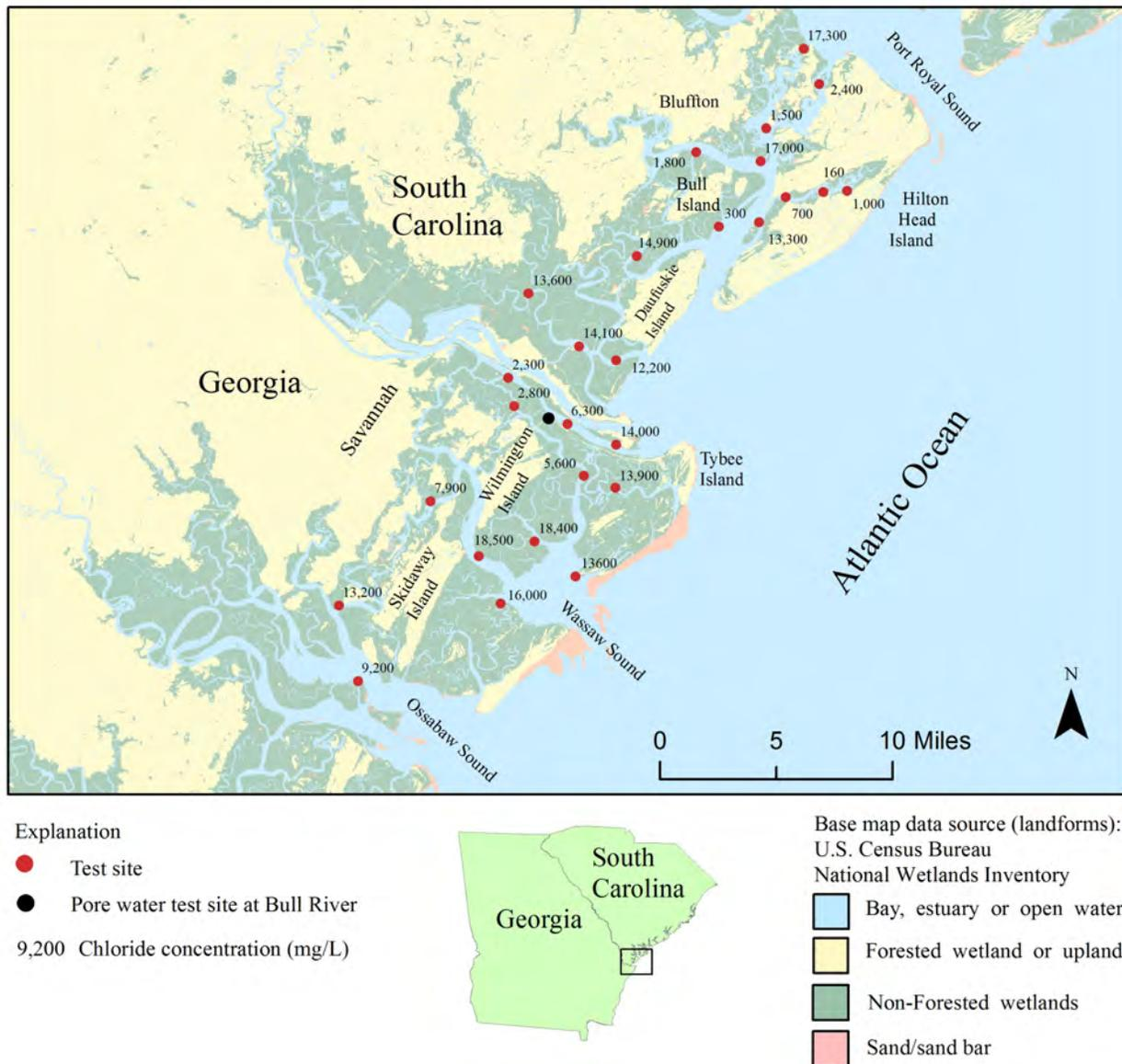
Figure 30. Test-boring locations and chloride concentrations near the bottom of the surficial aquifer between Port Royal Sound, S.C., and Ossabaw Sound, Ga. (Ransom and Park, 2011).
