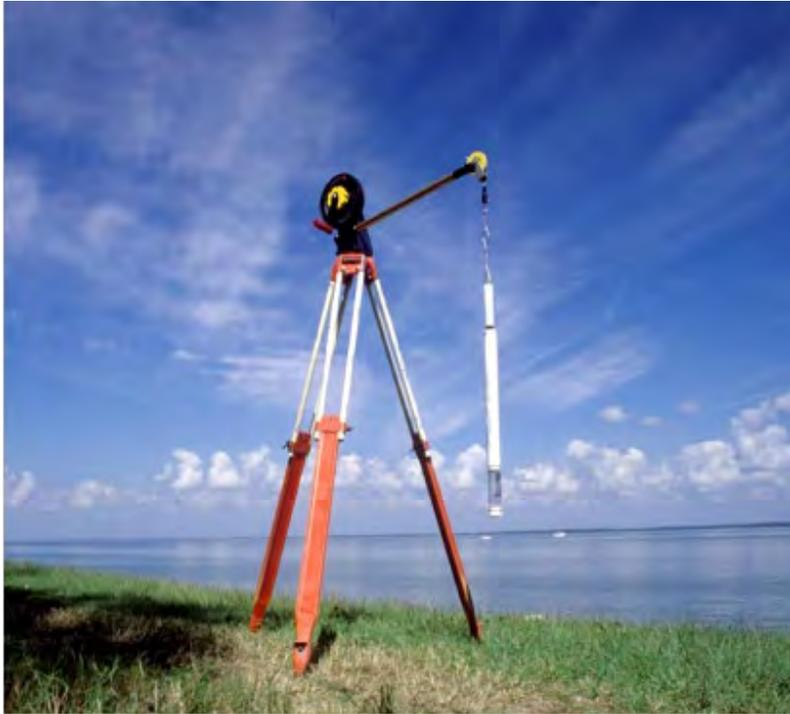
Downrigger with attached minisonde positioned on northern shore of Hilton Head Island with Port Royal Sound in background – equipment used to conduct vertical specific-conductance profiles in Upper Floridan wells aquifer. Photography by Camille Ransom, III.
