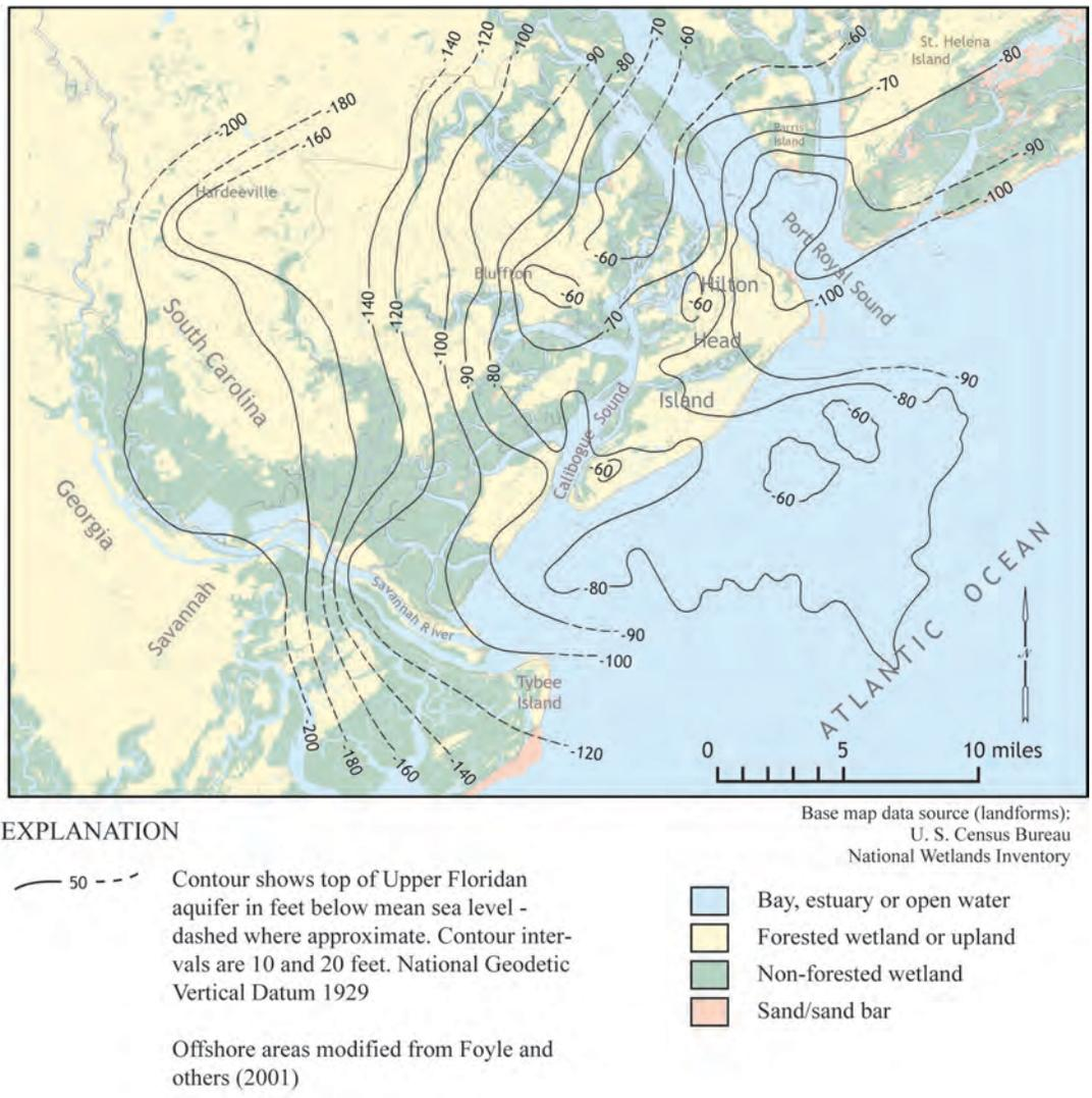
Figure 16. Structure contours for top of the Upper Floridan aquifer near Savannah, Ga., and Hilton Head Island, S.C.
