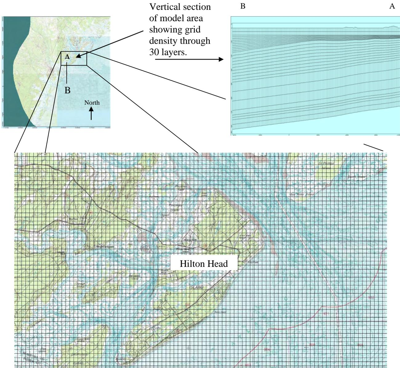
Figure J2. Map and section showing grid density for x, y, and z planes with  $\frac{1}{4}$  mi<sup>2</sup> cells, in part, for the model area in the vicinity of Hilton Head Island, S.C.
