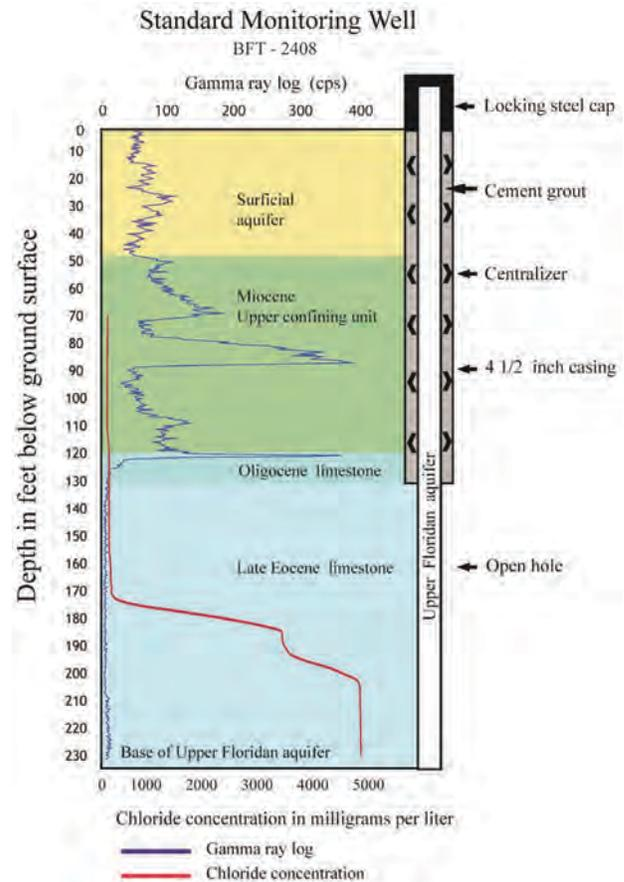
behind the grout and advanced by water pressure to the bottom of the well casing. Prior to advancing the borehole beneath the casing, measurements were taken inside the casing to determine if the grout had remained outside the casing. A 4.5-inch open borehole advanced to the bottom of the Upper Floridan aquifer completed the well (fig. 4).
