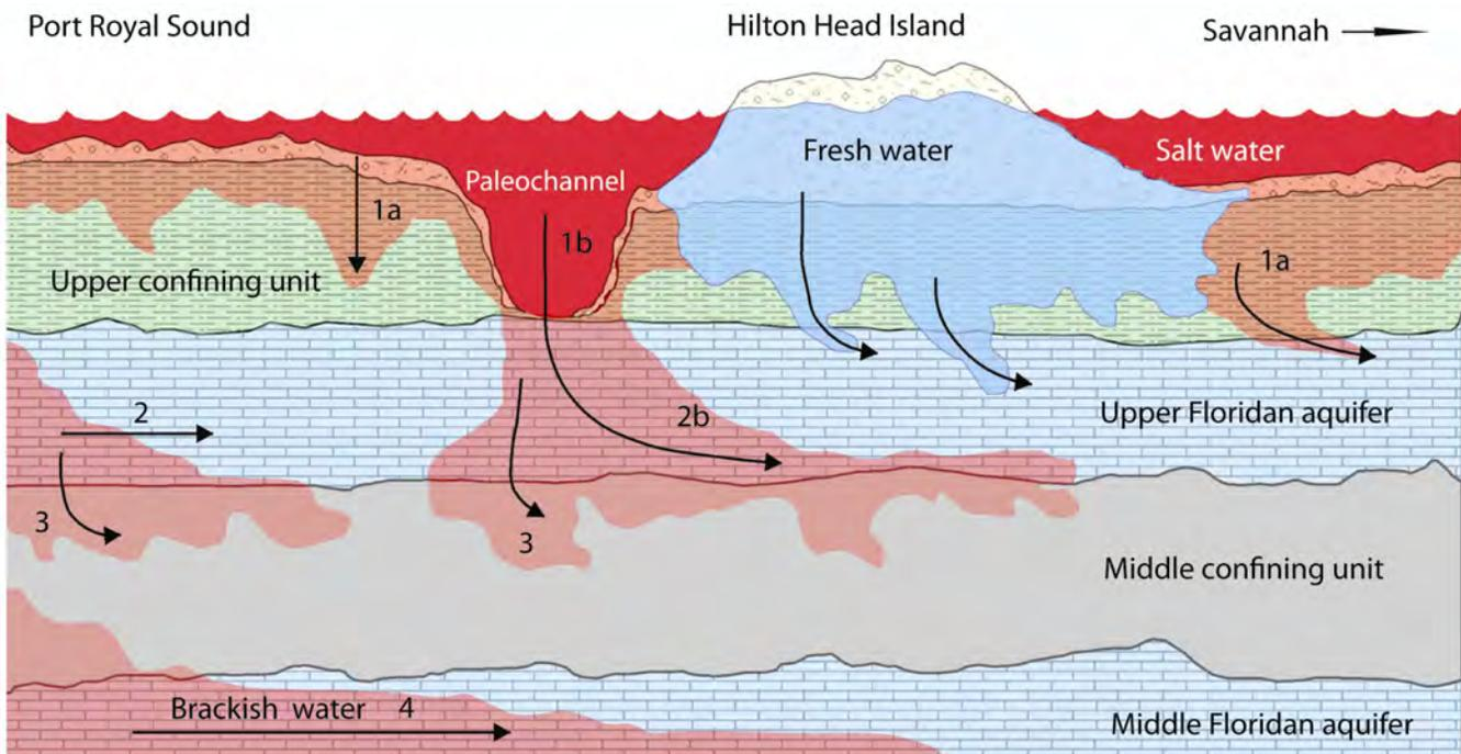
Figure 29. Generalized diagram showing saltwater movement in the Upper Floridan aquifer and adjacent confining units after groundwater withdrawals lowered the potentiometric head.
