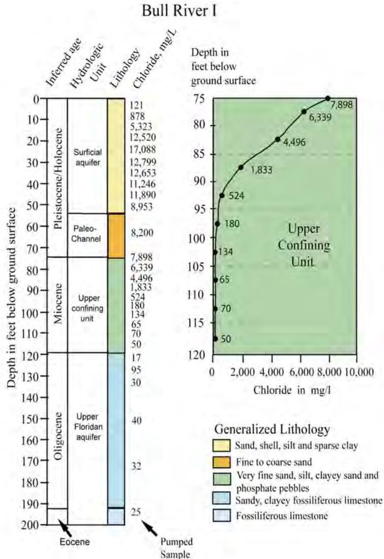
Figure 32. Chloride concentrations in pore-water samples from the surficial aquifer, upper confining unit, and Upper Floridan aquifer at well-site Bull River 1, 2005 (Ransom and others, 2006).
