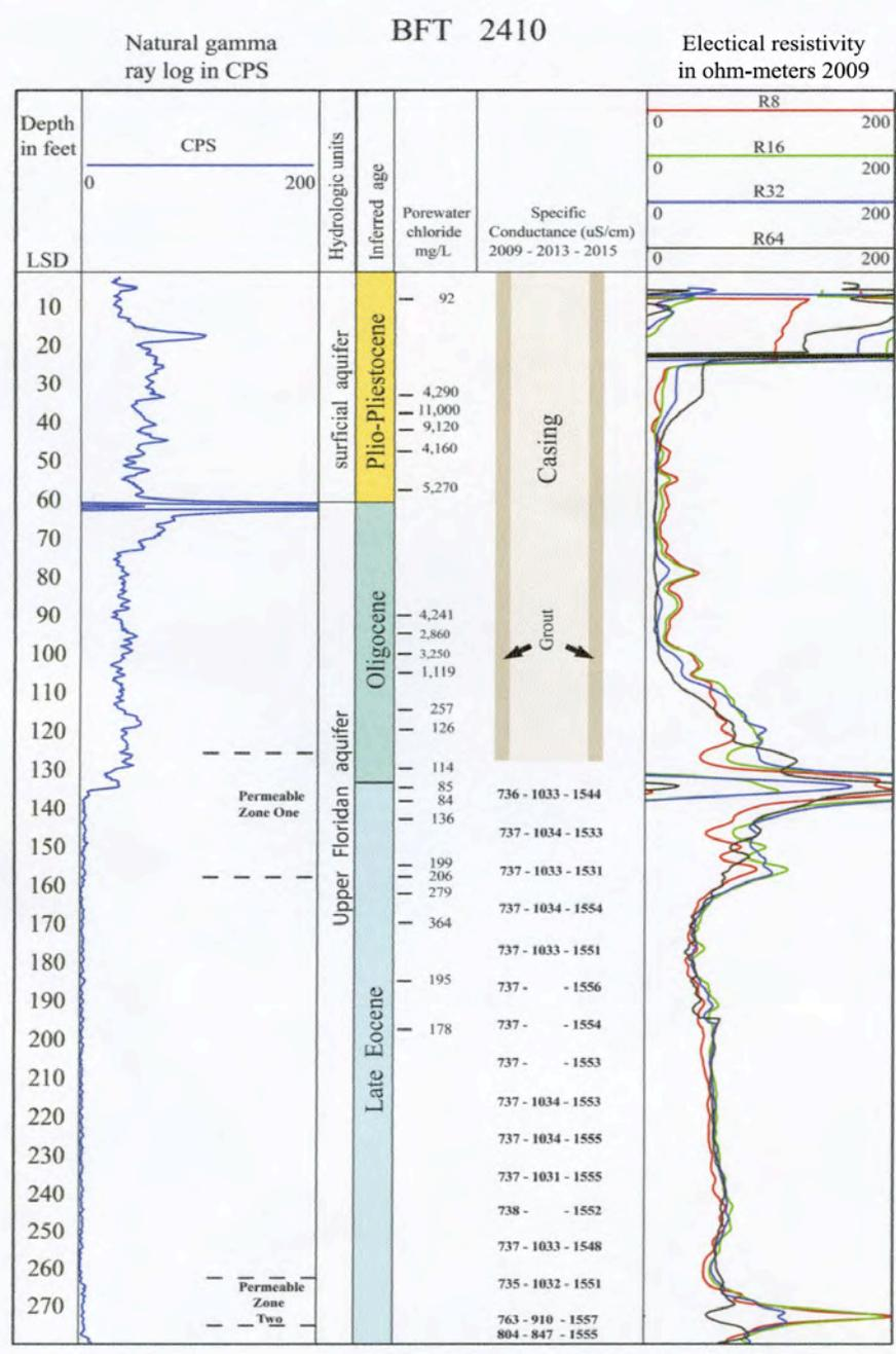
Figure 56. Hydrogeology, geophysical logs, specific-conductance profiles, chloride concentrations from pore-water, and well construction at well BFT-2410, Hilton Head Island, S.C., 2009–2015.
