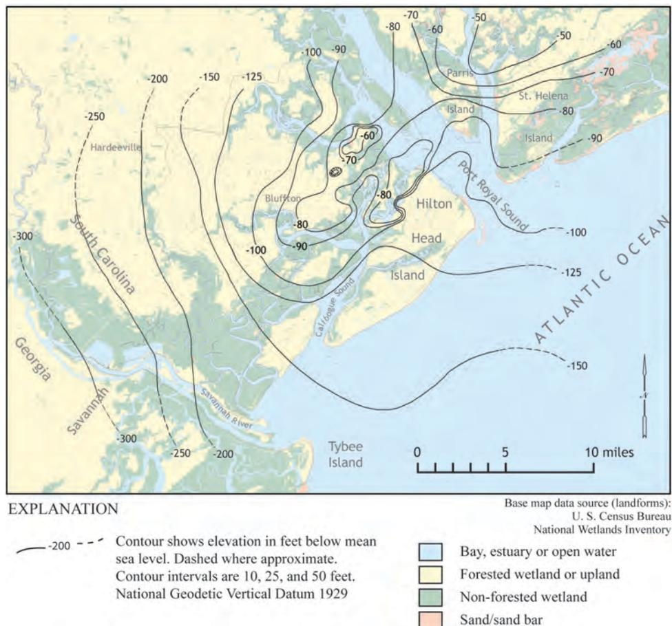
Figure 8. Structure contours showing top of the upper unit of the late Eocene Ocala Limestone near Savannah, Ga., and Hilton Head Island, S.C.
